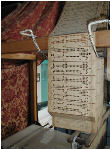
Figure 2. Punch cards used by a Jacquard loom, photographed at the Museum of Science and Industry, Manchester. The card sequence is an early material image of work as encoded variation.
